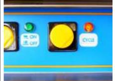
Press the Cycle button and the orange light will go on. You will hear the dishwasher in operation.
