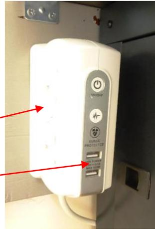
**1. Press the top button to switch on the power and the blue light will come on.**
